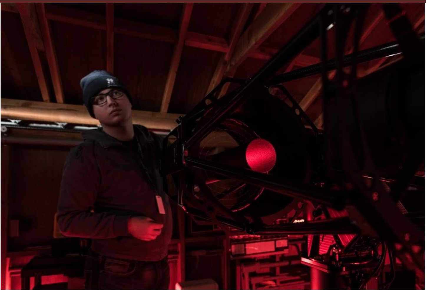
Dan working on the collimation of the Ritchey-Chretien telescope at the VCO, picture by Matt Watson
