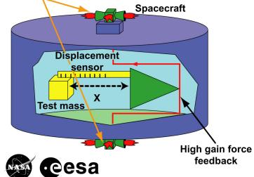
Space Technology 7 will test a technology to be used in detecting gravitational waves in space.
