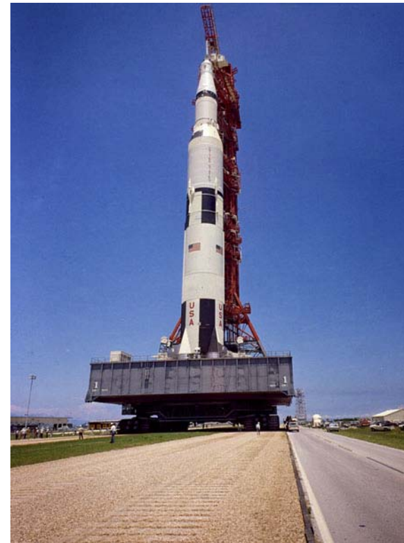
The Saturn V and Mobile Launch Platform are carried to the launch pad on the Crawler Transporter. Notice the tiny humans below the platform
